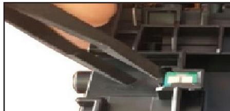
2. Use tweezers to remove the solder joint connecting the OEM cartridge and the chip.
