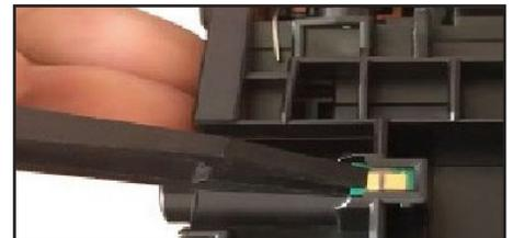
3. Clamp the OEM chip with tweezers and remove it in the direction of the red arrow.
