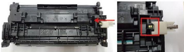
2. Push the metal blade as shown, ensuring that it touches the chip
