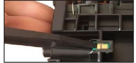
3. Install the chip as shown in the picture above. The printer will not recognize the toner cartridge if the chip is misaligned or facing the wrong direction.
