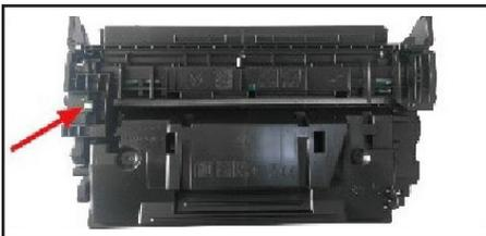
1. Remove the empty OEM cartridge from the printer and place it upside down on a table. Locate the chip position (as shown by the red arrow).
