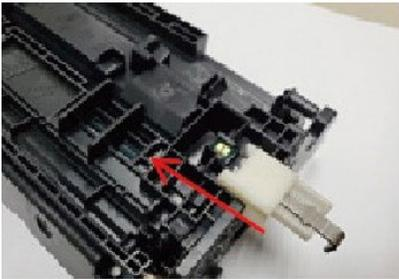
1. Locate the chip position and push the tailor-made tool into the bottom of the chip slot as shown.
