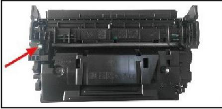
1. Carefully insert the chip into the chip slot of the new cartridge, making sure it is facing the correct direction as shown
