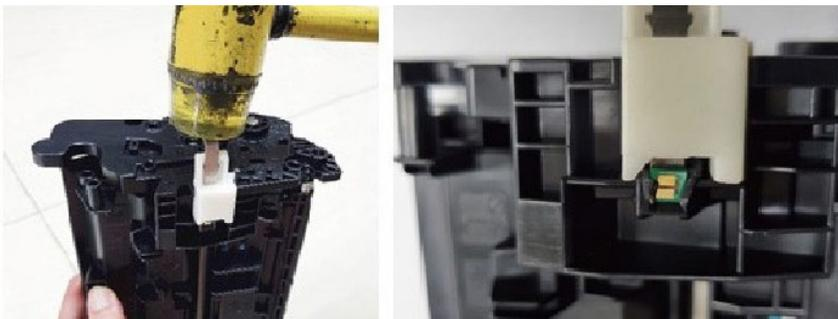
3. Hold the cartridge upright and position the tool upwards. Use a hammer to strike the end of the metal blade until the chip is completely separated from the chip slot, as shown.
